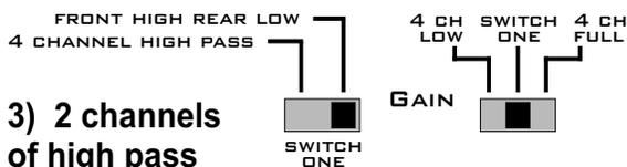
3) 2 channels of high pass and 2 channels of low pass.
