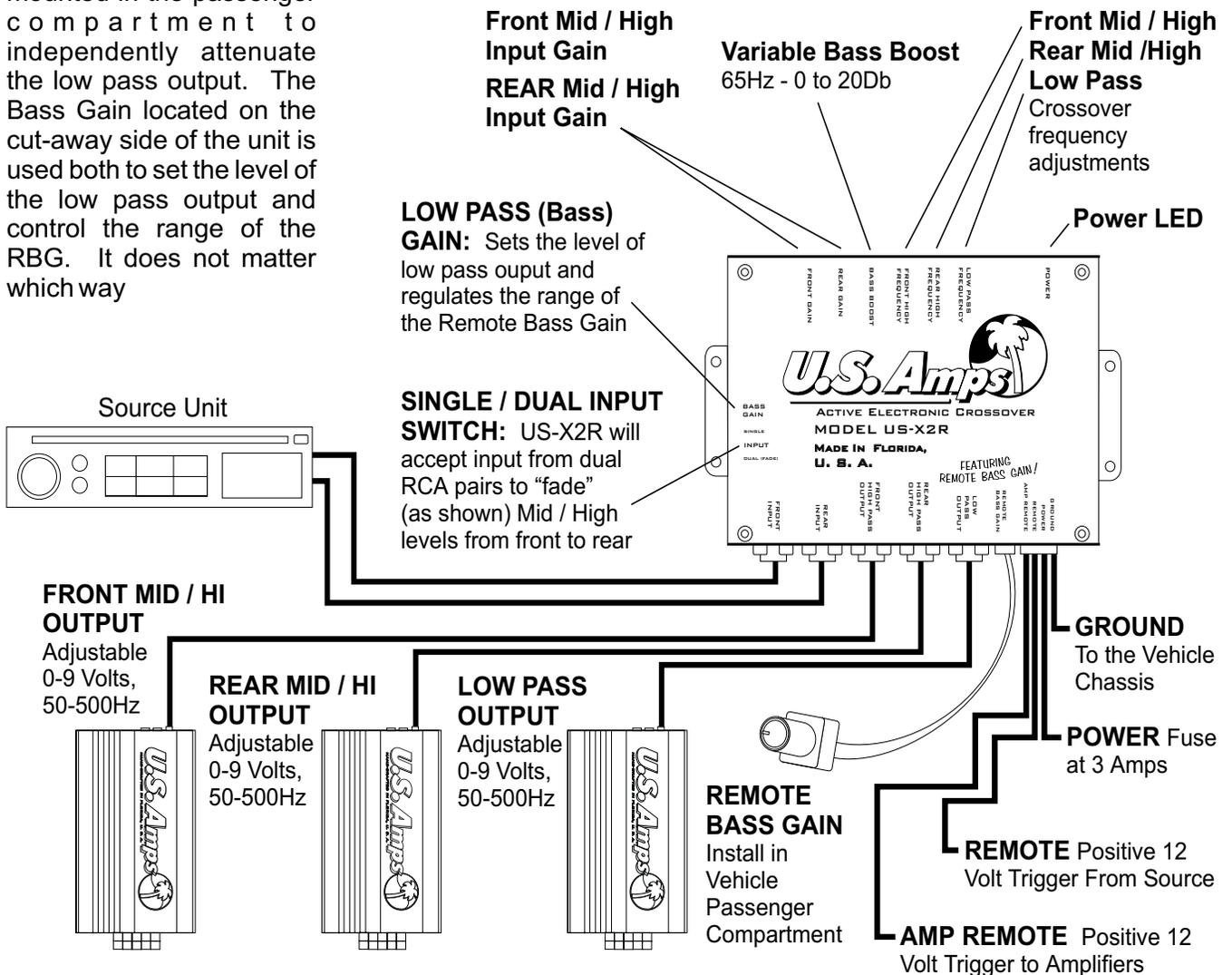
the RBG cable is connected. Use a common screwdriver tip or something like it to tighten the RBG knob.
