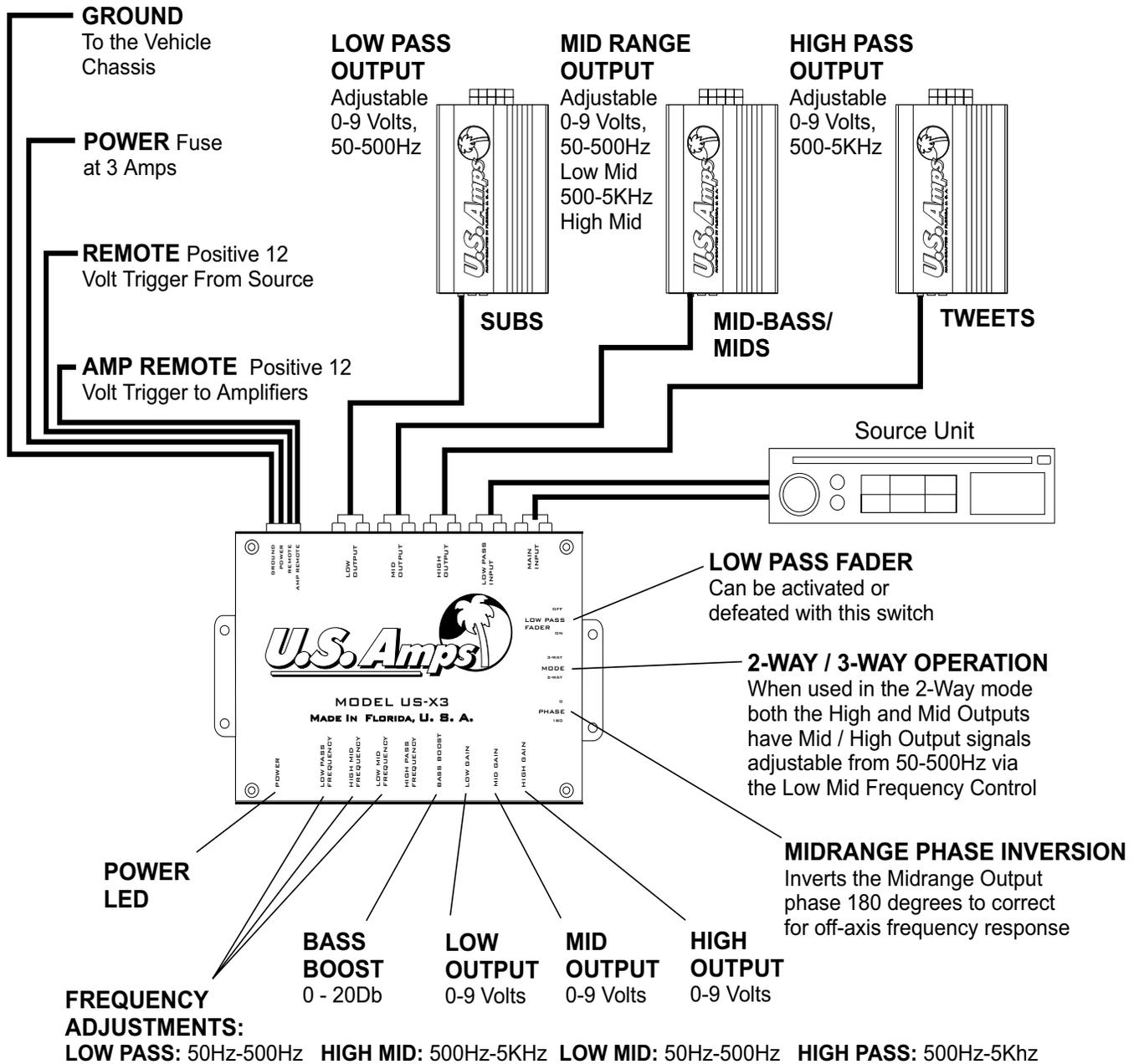
U.S. Amps crossovers feature an isolated input and amplifier section to keep the system free of noise. It is important to ground the crossover input for proper operation. Do not use a floating ground isolator with this or any other U.S. Amps product.
